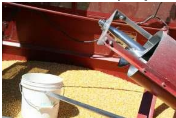
Fig. 2. Sampling corn for aflatoxin analysis in the experiments. The bucket is held under the auger as the combine moves through the plot so that only 10-11 lb. from a plot is sampled.
