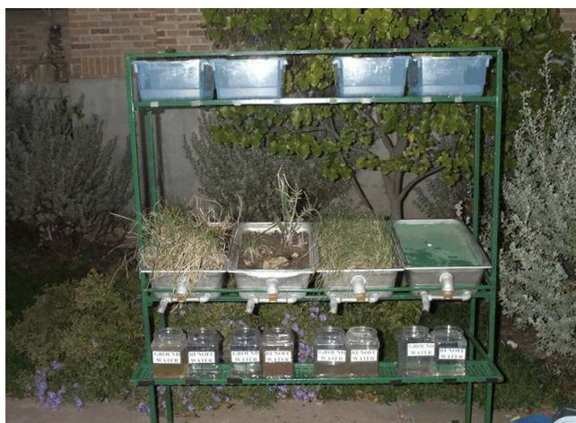
What is a Rainfall Simulator? A **rainfall simulator** simulates a rainfall event on a small specific area and allows water to either soak into the ground, through a porous soil layer and drain out the lower holes and into the container called “ground water”; or it runs off the top of the soil surface or impervious layer and out the top hole spilling into the container called “runoff water”.
