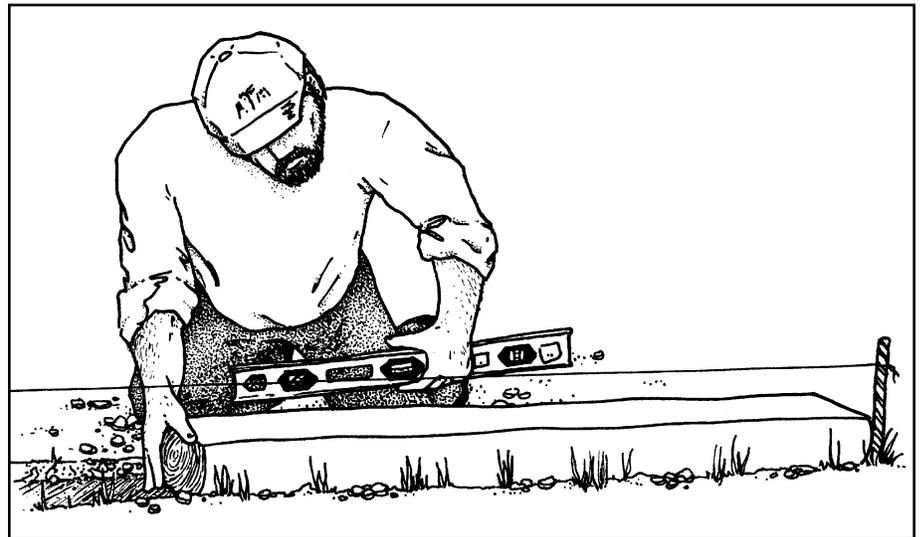
*Secure the first row of timbers by driving a piece of rebar through a predrilled hole and into the ground at a 20-degree angle. Secure subsequent rows with three or four spikes or pieces of rebar per timber. Make sure spikes extend well into the timber below.*
