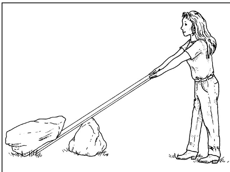
**Stone.** To raise the stones, roll them up a plank on pipes or use a hydraulic lift. To install a dry stone wall, first level the terrain of the perimeter. Lay the stones in
