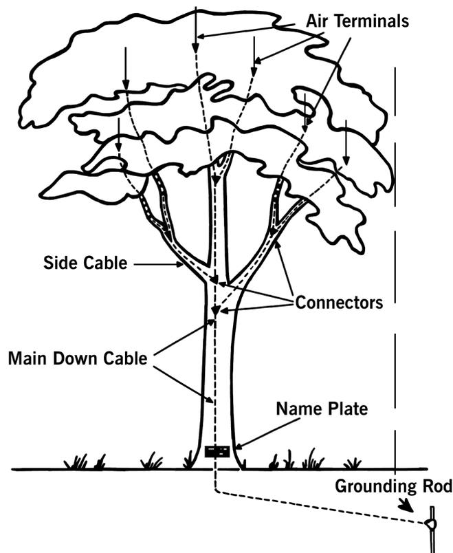
**Figure 4. Tree with properly installed lightning protection system.**
