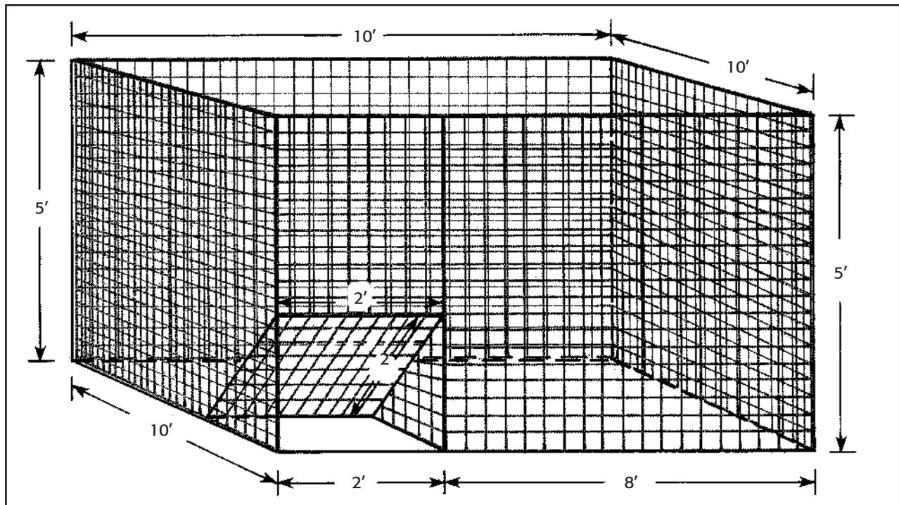
Figure 3. Multi-catch live trap for feral hogs.
