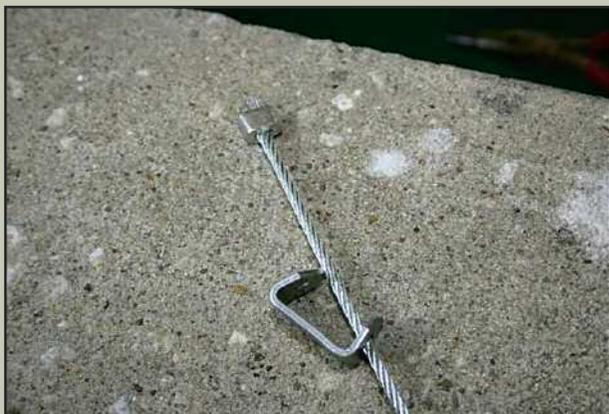
**Run the cable through the snare lock.**
