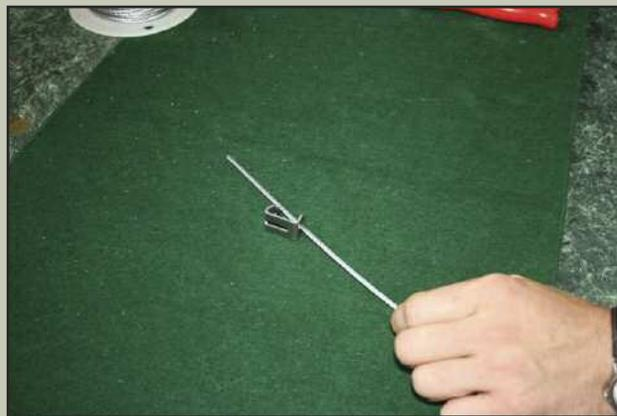
**Run the cable through the snare lock.**
