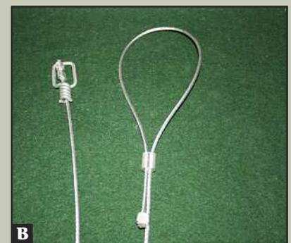
**Attach a ferrule to the end of the cable (A). The snare can be designed with a swivel end (B-left) or an adjustable end (B-right).**
