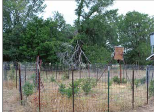
Figure 10. Remotely triggered trap gates use motion sensing cameras to capture real time activity and images at trap sites. The trapper can close the door at their discretion using a mobile phone or computer.
