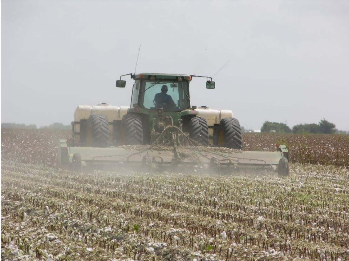
**"Notice the Shredder is equipped to spray behind it."**
