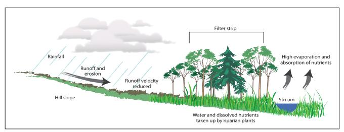
Figure 11. Conceptual model of how vegetative filter strips protect a stream from contaminants and the riparian area from erosion. Illustration by Jennifer Peterson.
